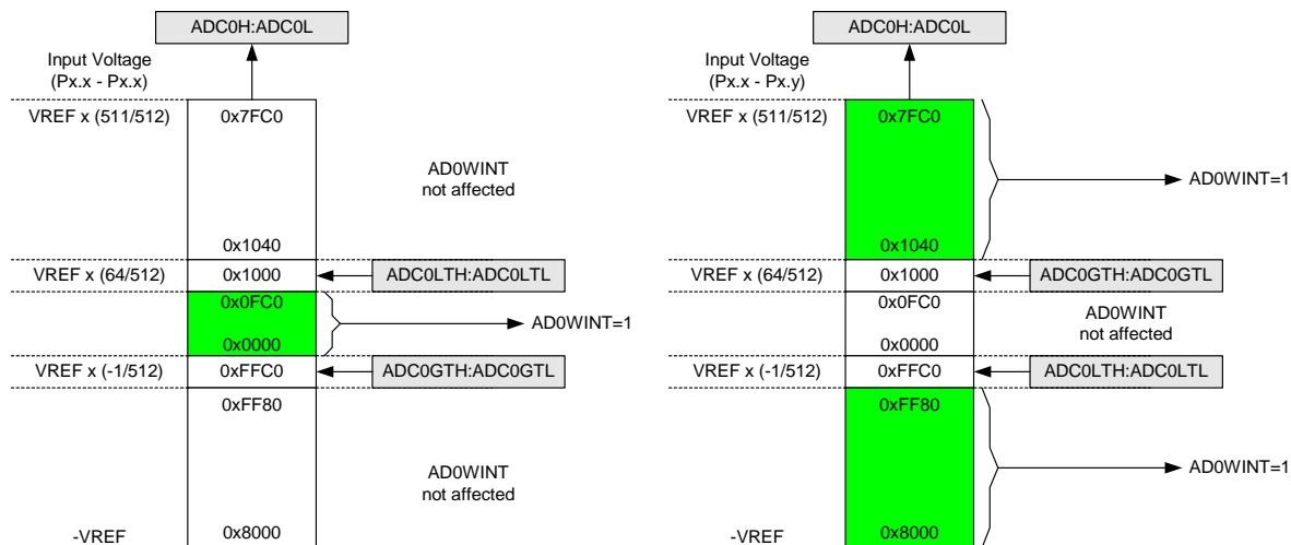
Figure 5.8. ADC Window Compare Example: Left-Justified Differential Data
