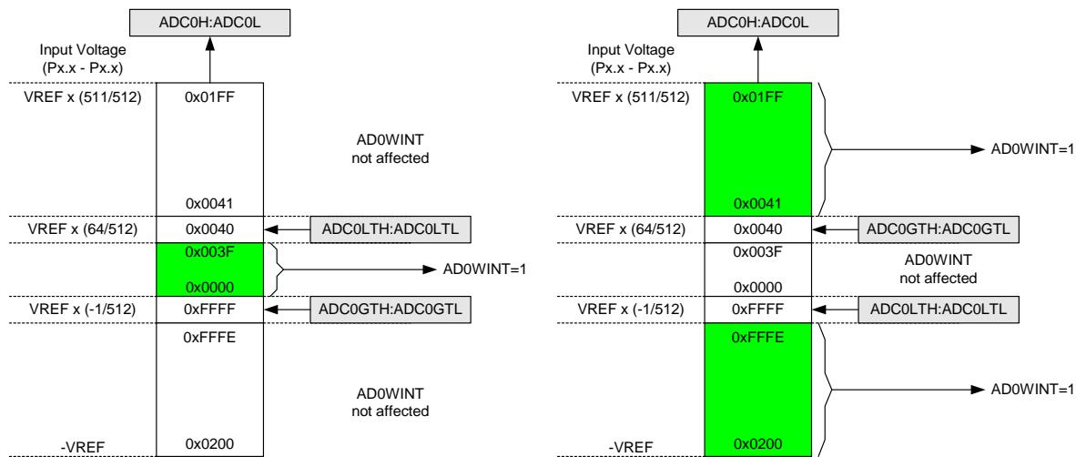
Figure 5.7. ADC Window Compare Example: Right-Justified Differential Data
