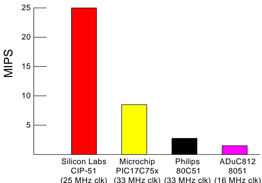
Figure 1.7. Comparison of Peak MCU Execution Speeds
