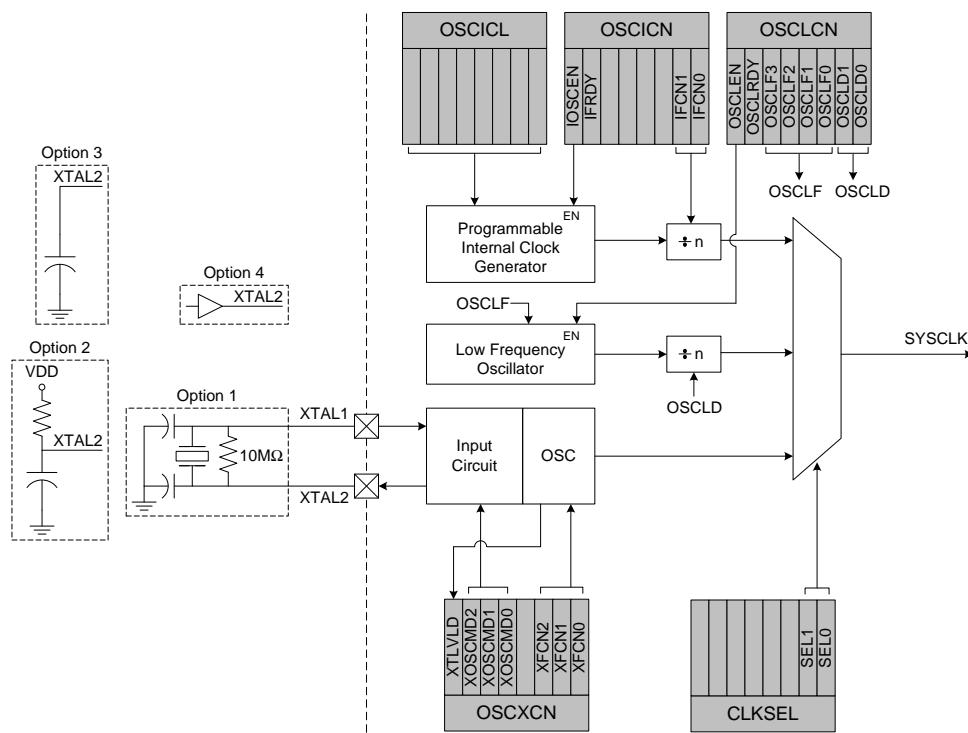
**Figure 13.1. Oscillator Diagram**
