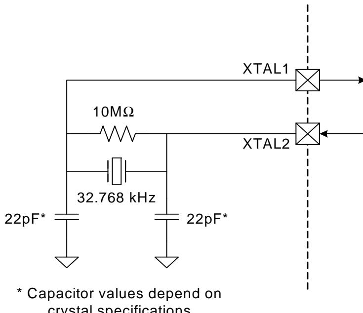
**Figure 13.2. External 32.768 kHz Quartz Crystal Oscillator Connection Diagram**
