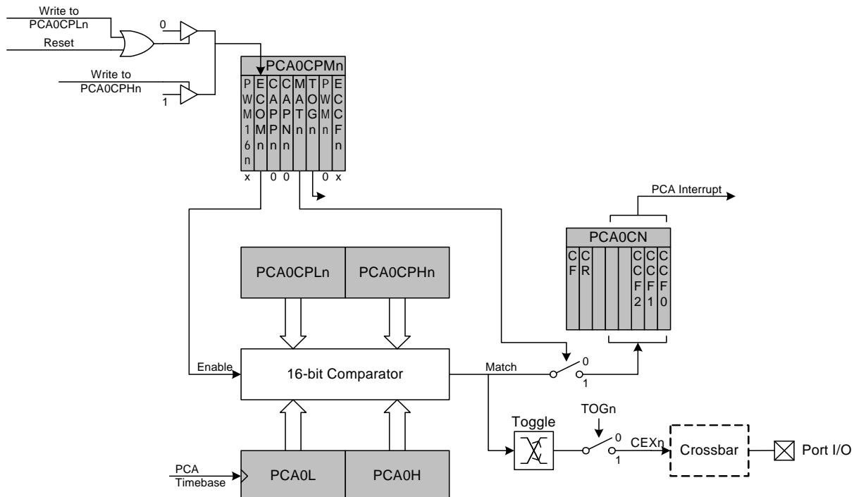
Figure 19.6. PCA High-Speed Output Mode Diagram
