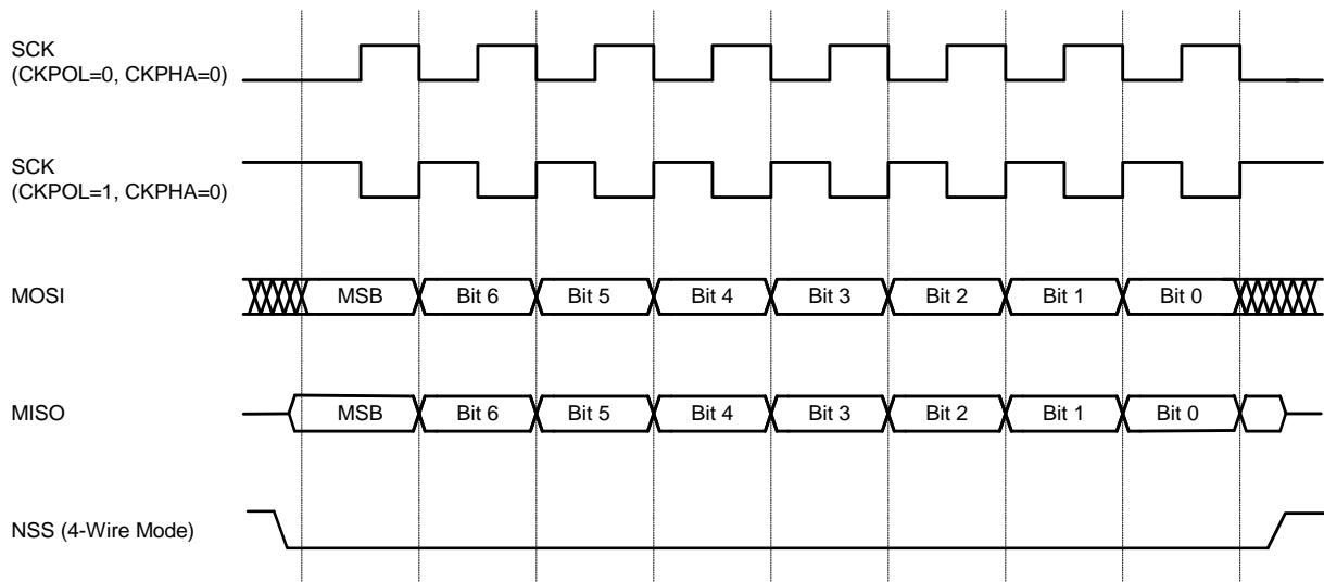
**Figure 17.6. Slave Mode Data/Clock Timing (CKPHA = 0)**
