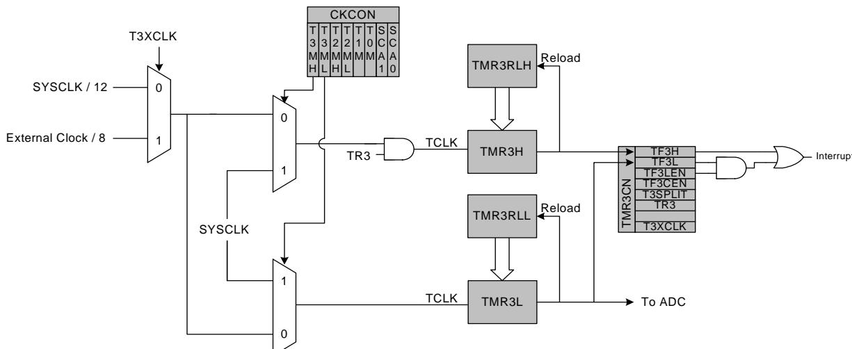
Figure 18.7. Timer 3 8-Bit Mode Block Diagram
