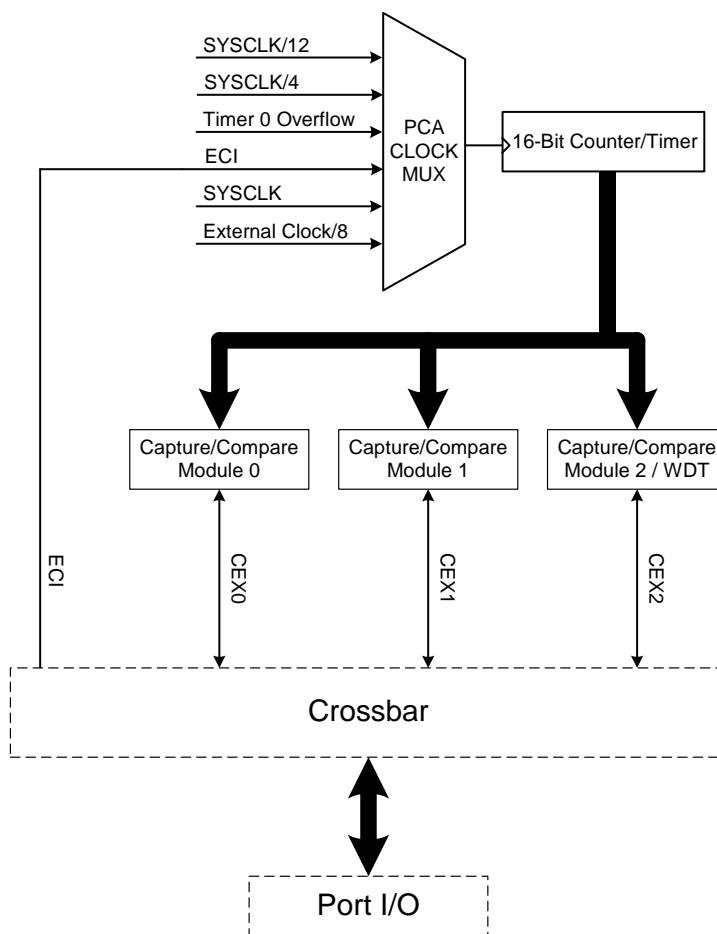
Figure 19.1. PCA Block Diagram
