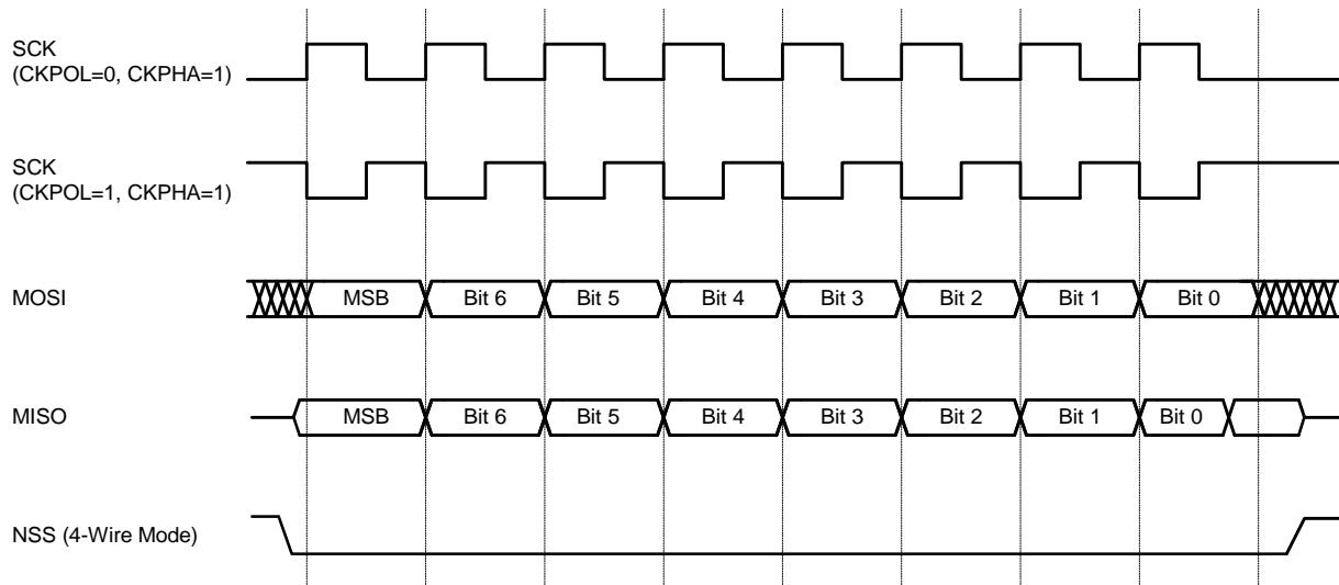
**Figure 17.7. Slave Mode Data/Clock Timing (CKPHA = 1)**
