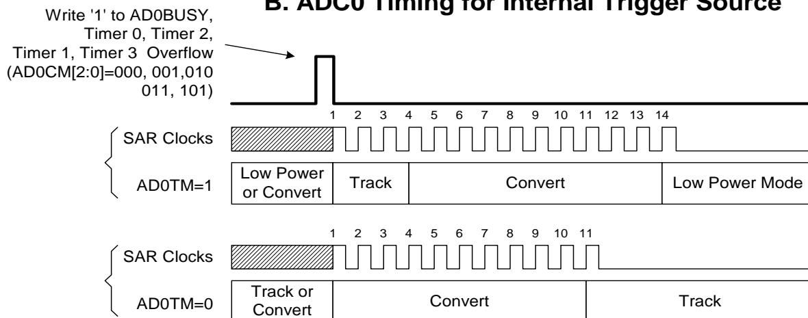
**Figure 5.3. 10-Bit ADC Track and Conversion Example Timing**
