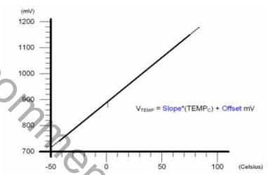
Figure 6.2. Typical Temperature Sensor Transfer Function
