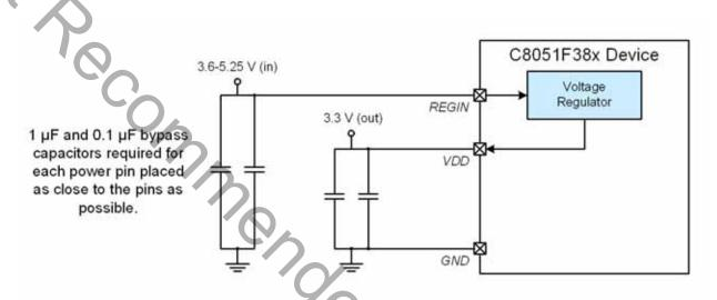
Figure 4.1. Connection Diagram with Voltage Regulator Used
