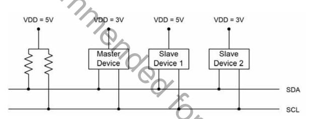
Figure 21.2. Typical SMBus Configuration
