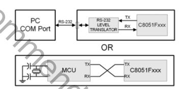
Figure 23.5. Typical UART Interconnect Diagram
