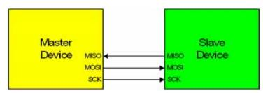
Figure 24.3. 3-Wire Single Master and 3-Wire Single Slave Mode Connection Diagram
