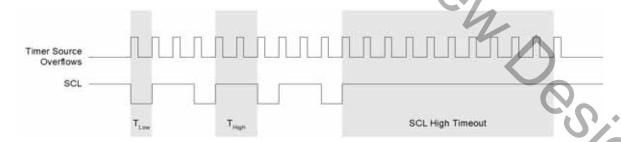
Figure 21.4. Typical SMBus SCL Generation
