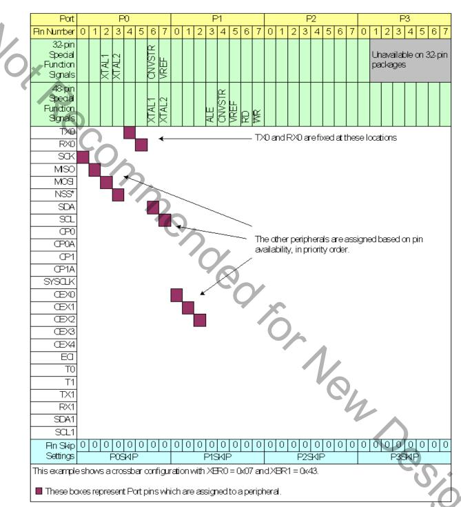
Figure 20.4. Crossbar Priority Decoder in Example Configuration (No Pins Skipped)
