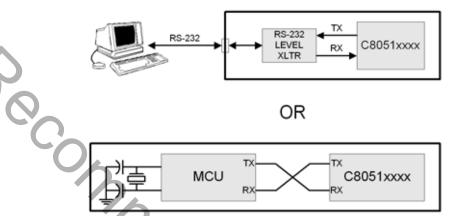
Figure 22.3. UART Interconnect Diagram
