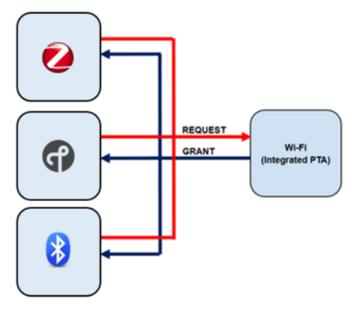
Figure 4-3. Three EFR32s Supporting Single Wi-Fi 2-Wire PTA Interface (REQUEST pull-up or pull-down not shown)
