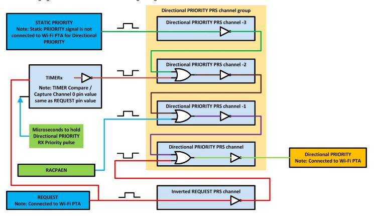
Figure 4-11. EFR32xG1x Directional PRIORITY Logic Diagram
