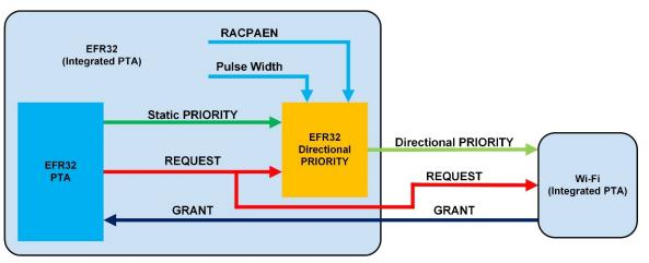
Figure 4-9. Single-EFR32 PTA without SDK PWM, with Directional PRIORITY
