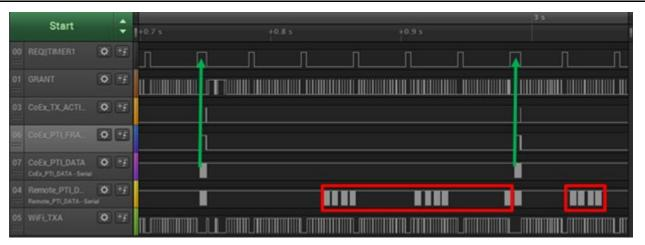
Figure 4-6. EFR32 RX Success with PWM during High-Duty Cycle Wi-Fi TX
