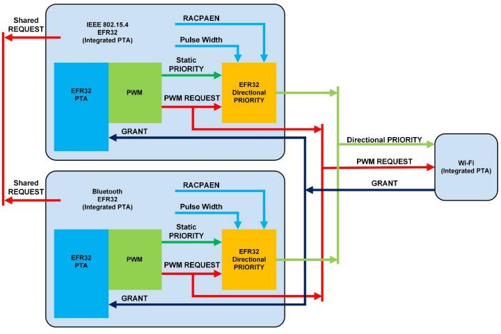
Figure 4-10. Multi-EFR32 PTA with SDK PWM and Directional PRIORITY (1K 5% pull-ups and pull-downs not shown)
