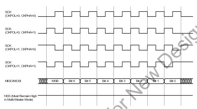
Figure 25.5. Master Mode Data/Clock Timing
