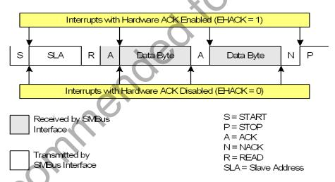
Figure 26.6. Typical Master Read Sequence
