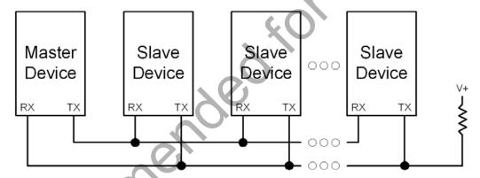
Figure 27.6. UART Multi-Processor Mode Interconnect Diagram
