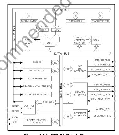
Figure 14.1. CIP-51 Block Diagram
