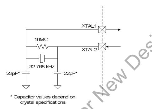
Figure 22.2. External 32.768 kHz Quartz Crystal Oscillator Connection Diagram
