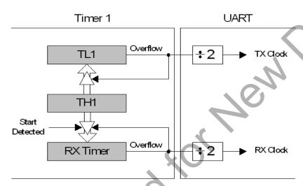
Figure 27.2. UARTO Baud Rate Logic
