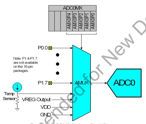
Figure 8.6. ADC0 Multiplexer Block Diagram
