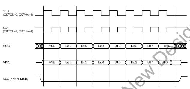
Figure 25.7. Slave Mode Data/Clock Timing (CKPHA = 1)
