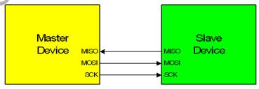
Figure 25.3. 3-Wire Single Master and 3-Wire Single Slave Mode Connection Diagram
