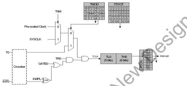
Figure 28.1. T0 Mode 0 Block Diagram
