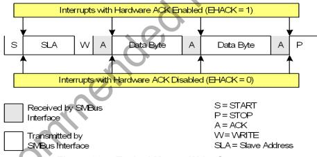
Figure 26.5. Typical Master Write Sequence
