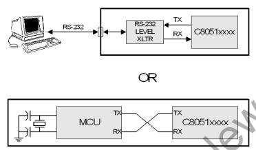
Figure 27.3. UART Interconnect Diagram
