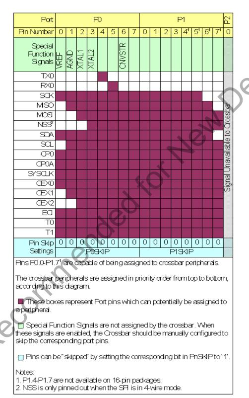
Figure 23.4. Priority Crossbar Decoder Potential Pin Assignments
