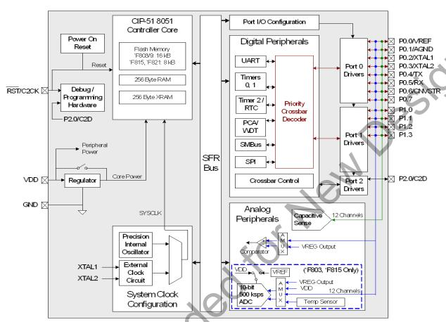
Figure 1.4. C8051F803, C8051F809, C8051F815, C8051F821 Block Diagram
