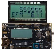
3. Additionally, the display has a feature called charge redistribution, which can be used to reduce the power consumption of the display at the cost of lower display contrast. To enable or disable charge distribution, press the pushbutton [**BTN0**] on the kit.
