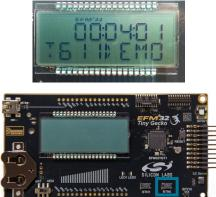
4. The second screen displays the intensity of the magnetic field, in mT, near the Silicon Labs Si7210 Hall Effect sensor, mounted on the bottom-right of the kit. Placing a magnet near this sensor will update the display with the strength of the field.
