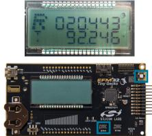
6. The fourth screen shows data coming from the capacitive sense slider. The EFM32TG11 Tiny Gecko has an advanced SAR-based capacitive touch peripheral with up to 64 inputs that provides the touch measurements. The top line of the display, next to "F", displays the force of the capacitive touch, while the line next to "POS" displays the position of the touch on the slider, from 0 to 64, from left to right.
